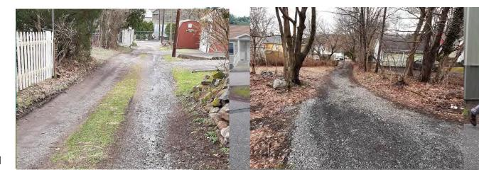
The alleyway between Washington Avenue and Elm Street can be converted to a pervious pavement road. It will capture and infiltrate the nearby stormwater runoff from Washington Avenue, Elm Street, and the adjacent properties.
