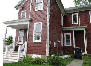
Two rain gardens can be used to capture, treat, and infiltrate rooftop runoff. A downspout planter box can be constructed along the building to allow roof runoff to be captured and reused. A preliminary soil assessment suggests that the soils have suitable drainage characteristics for green infrastructure.
