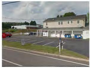
Areas of the parking lot can be retrofitted with porous pavement to capture stormwater runoff from the parking lot. A preliminary soil assessment suggests that the soils have suitable drainage characteristics for green infrastructure.
