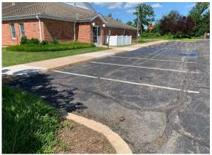
A bioretention system can be installed on the west side of the building to help infiltrate the stormwater from four downspouts. Pervious pavement can be installed in the south parking lot to capture the stormwater runoff from the lot. A preliminary soil assessment suggests that more soil testing would be required before determining the soil's suitability for green infrastructure.
