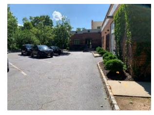
Pervious pavement can be installed in the eastern parking lot to capture, treat, and infiltrate the stormwater from the parking lot. A bioretention system can be installed on the northern side of the building to capture stormwater runoff from the north section of the parking lot. A preliminary soil assessment suggests that the soils have suitable drainage characteristics for green infrastructure.
