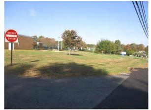
Two rains gardens can be installed in the turfgrass in front of the building to capture, treat, and infiltrate roadway runoff. Another rain garden can be installed south of the building to capture runoff from the basketball court. Pervious pavement can be installed in the parking lot to capture and infiltrate stormwater runoff from the parking lot. A preliminary soil assessment suggests that more soil testing would be required before determining the soil's suitability for green infrastructure.
