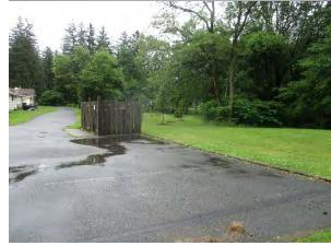
Pervious pavement can be installed in the western corner of the parking lot to capture and infiltrate stormwater runoff from the parking lot. A rain garden can be installed along the roadway south of the building to capture stormwater runoff from the pavement. A preliminary soil assessment suggests that more soil testing would be required before determining the soil's suitability for green infrastructure.
