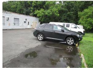
Porous pavement can be installed in the parking lot to capture stormwater from the building and parking lot to alleviate flooding issues as seen in the image above. A preliminary soil assessment suggests that the soils have suitable drainage characteristics for green infrastructure.
