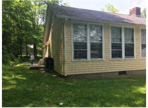
A rain garden can be installed in the turfgrass area on the east side of the building to capture, treat, and infiltrate stormwater runoff from the roof. Downspout planter boxes can be installed to allow roof runoff to be captured and reused. A preliminary soil assessment suggests that the soils have suitable drainage characteristics for green infrastructure.
