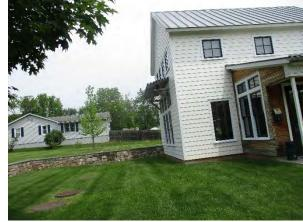
A rain garden can be installed in the turfgrass area to capture, treat, and infiltrate stormwater runoff from the roof. Downspout planter boxes can be constructed along the building to allow roof runoff to be captured and reused. A preliminary soil assessment suggests that more soil testing would be required before determining the soil's suitability for green infrastructure.
